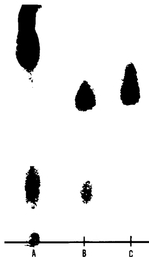
Figure 2. Positive print made from a contact negative of a glass-paper chromatogram showing the chromatographic identification of the principal phospholipides in sugar cane juice
